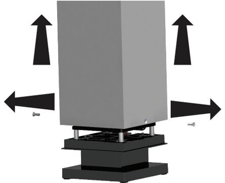
1. Remove two (2) screws at the bottom sides holding outer shell in place. Then slide the shell up and off of the internal base.
